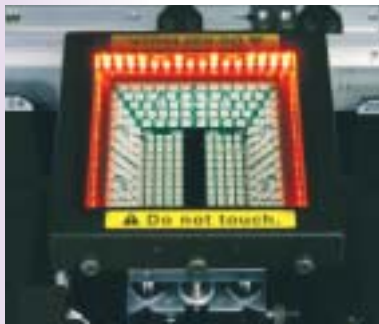
BGA image with side illumination on line array camera
